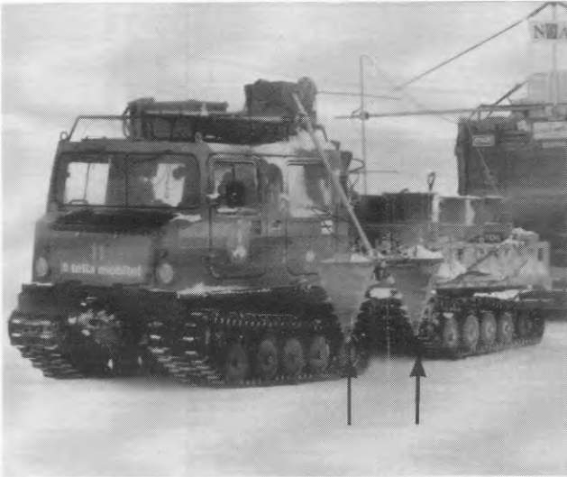
Figure 2. The snow radar antennae (indicated by arrows) were mounted on a steel frame on an all terrain carrier. The radio-echo sounder was installed inside the vehicle.
